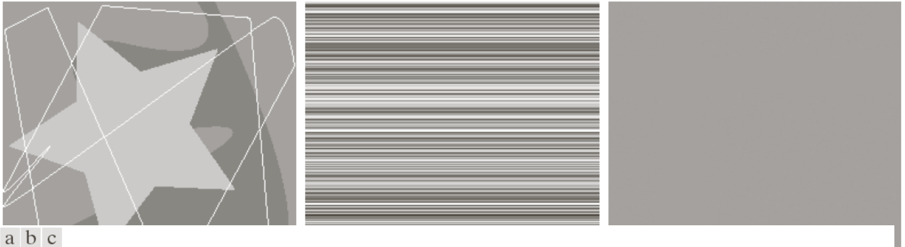
FIGURE 8.1 Computer generated 256 \times 256 \times 8 bit images with (a) coding redundancy, (b) spatial redundancy, and (c) irrelevant information. (Each was designed to demonstrate one principal redundancy but may exhibit others as well.)
